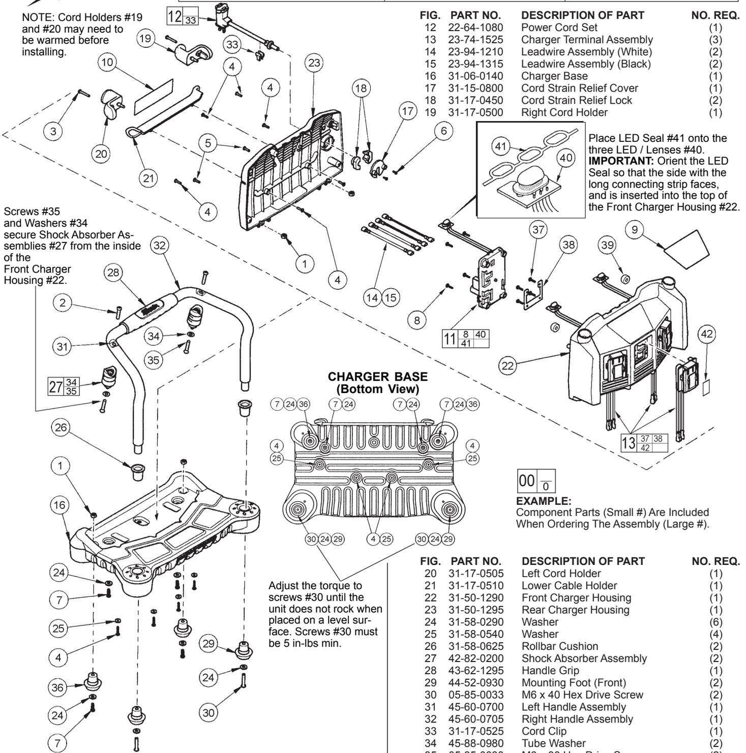
Screws #35 and Washers #34 secure Shock Absorber Assemblies #27 from the inside of the Front Charger Housing #22.
