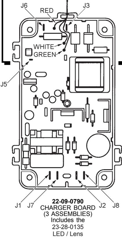
Place the **first** charger board in the middle, lower position (bay 2). Place the other two charger boards into bays 1 & 3.
