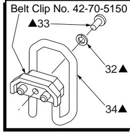
There are 2 belt clip designs for this tool. The initial design, Belt Clip #34, 42-70-5150 is being discontinued and replaced by Belt Clip Assembly #80, 42-70-2653.
