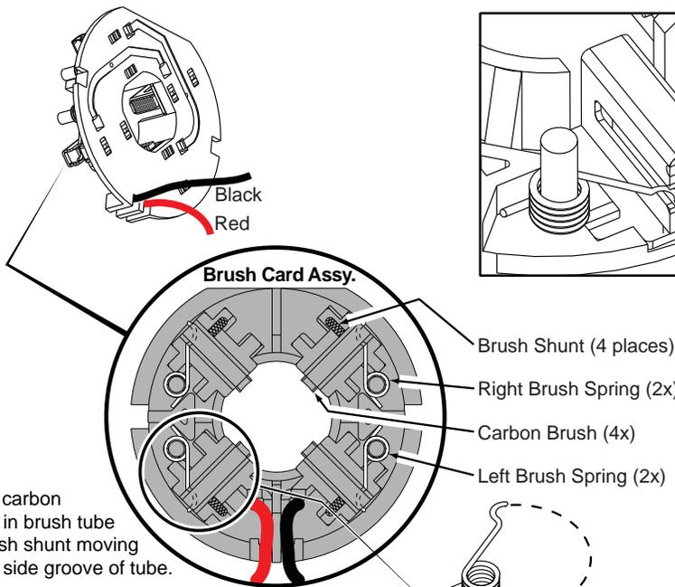
Be sure carbon brush is in brush tube with brush shunt moving freely in side groove of tube.
