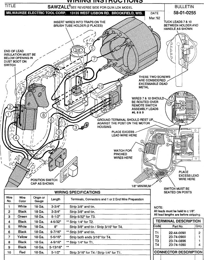
\*\* = Component of switch module assembly.
