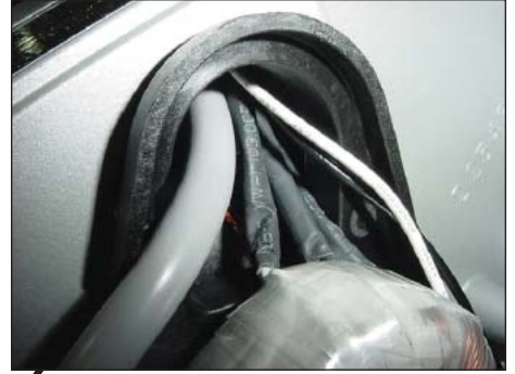
Opening for wires and harnesses as viewed from the other side of the Motor Arm Assembly.
