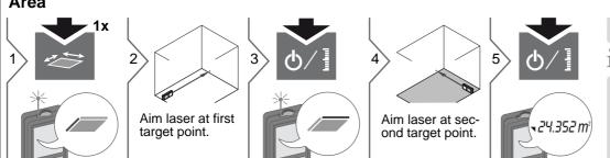
The result is shown in the main line and the measured value above.
