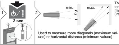
The minimum and maximum distance measured is displayed max. (min, max.). The last value measured is displayed in the main line.
