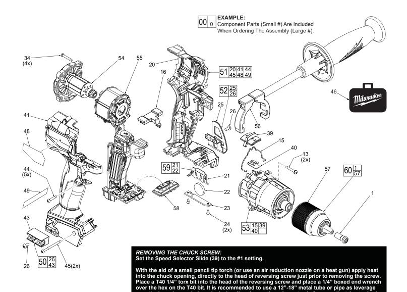
over the boxed wrench. In a clockwise direction apply a slow, steady force on the 'cheater bar'
