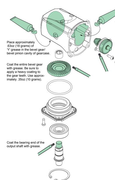
Place approximately .70oz (20 grams) of 'Y' grease in the gearcase cavity for the armature pinion and intermediate gear assembly.
