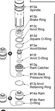
Prior to installing internal spindle components, lightly grease the inside cavity of spindle.
