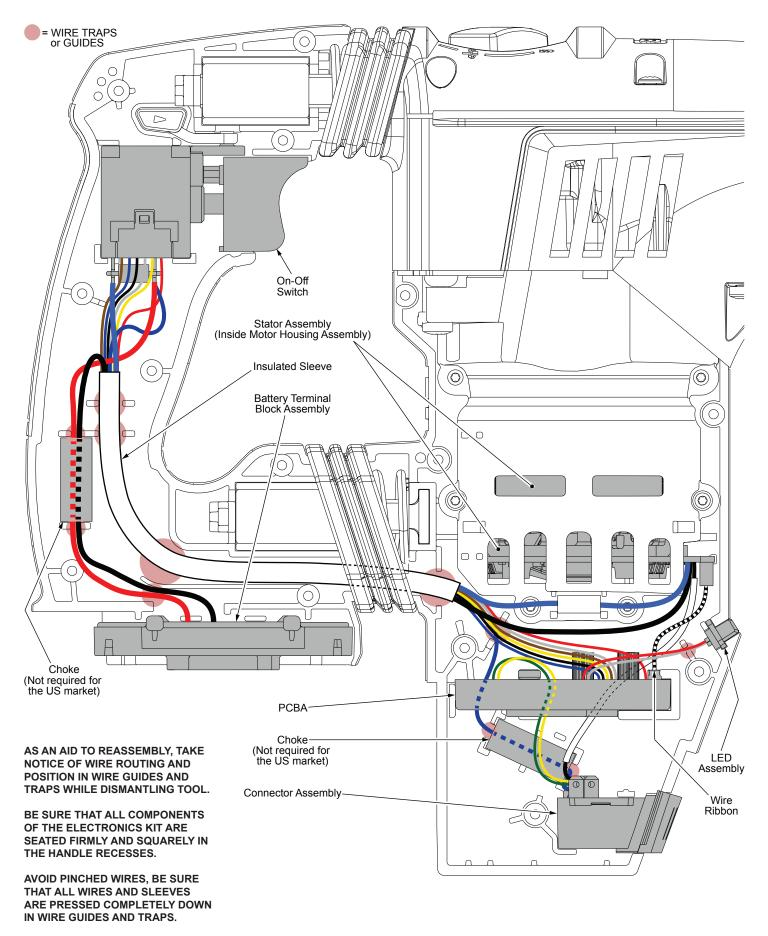
PRIOR TO INSTALLING THE HANDLE COVER ONTO THE HANDLE SUPPORT, BE SURE THAT THERE ARE NO INTERFERENCES.
