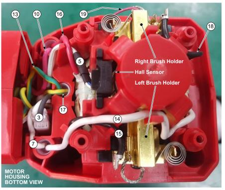
BLK & WHITE From Control Board. Both black and white wires are terminated together. Connect with black & white wires from EM clutch.
