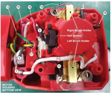
3 BLK & WHITE From Control Board. Both black and white wires are terminated together. Connect with black & white wires from EM clutch.
