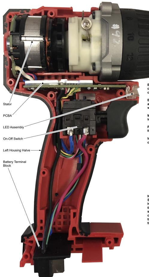
Be sure that all mechanical and electrical components are placed firmly and squarely in corresponding cavities of left housing halve.
