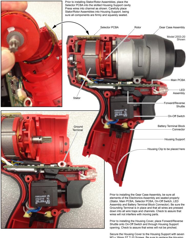
M3 x 16mm ST T-10 Screws. Be sure to replace the Housing Clip at the bottom of the battery opening.
