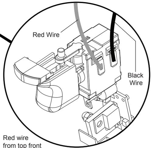
Red wire from top front position on switch to left brush card position (marked with an 'L').
