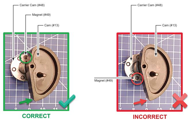
The magnet is on the opposite end from the pointed end of the cam. This is the correct position.
