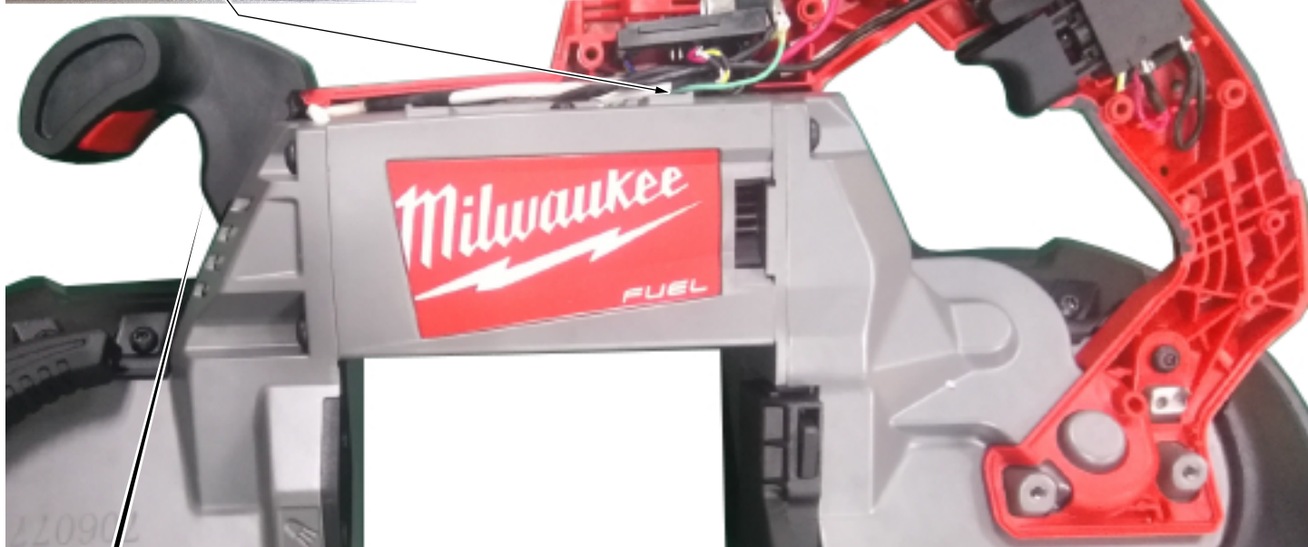
Bottom of T-Handle showing Micro-Switch wire routing
