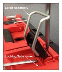
Pins to be installed from the inside of the handle.
