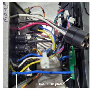
Make sure that no wire crosses over this blue wire when fastening the small PCB plate.
