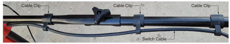
Secure the Switch Cable with three Cable Clips, as shown.
