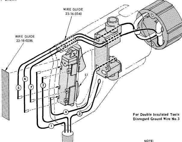
Refer to electrical parts chart for terminal and connector part nos. and quantity required - see drawing for actual hook-up.
