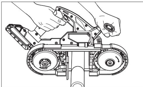
3. To vary the speed, increase or decrease pressure on the rear handle trigger. The further the trigger is pulled, the greater the speed.
