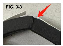
3. Apply small amount of glue to one end of seal, coating evenly (FIG. 3-1). Align and press the ends together, holding for at least 5 seconds to ensure adhesion. Verify ends are aligned and attached. (FIG. 3-2 is correct, FIG. 3-3 is incorrect.)
