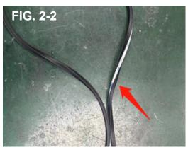
2. Remove seal and unroll. Make sure seal is not twisted. (FIG. 2-1 is correct, FIG. 2-2 is incorrect).
