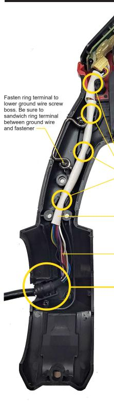
Place switch wire above handle mounts with excess wire loop between screw bosses
