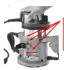
break-the-edge — sand entire inside edges of milled slot and upper & lower circumferences of motor section of base, as shown, to eliminate burr and possible binding condition
