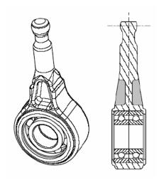
**14-67-0135 Wobble Plate Assembly** is a new service replacement part for the primary wobble plate used in the 6509-20, 6509-22 Sawzall $^{\$}$ , 6519-22 Sawzall Plus $^{\$}$ .
