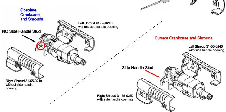
Use Crankcase 28-14-2295 when servicing a Rotary Hammers 5316 and 5316-4
