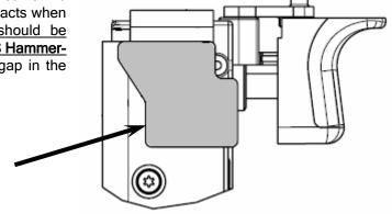
To reduce high vibration loads to internal switch contacts the rubber spacer is required when installing the -1779 Switch into a 0779-20, 0779-50 or 0799-20 1/2" V28 Impact Wrench.
