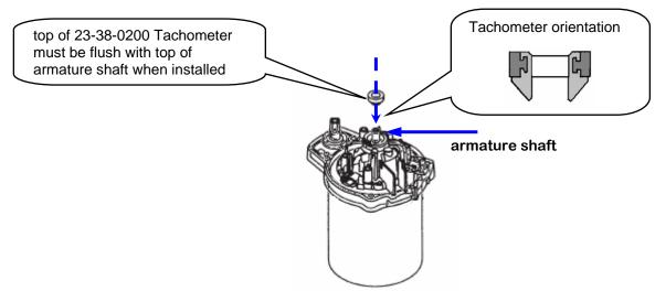
tachometer must be installed flush to the top of the armature shaft and in the proper orientation; if installed incorrectly tool's speed and performance will be compromised note: tachometer can be pushed sub-flush on shaft of Router armature
