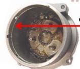
Gearcase has machined undercut
