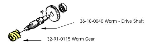
Please Note! 36-18-0040 Worm Gear Shaft is 'OBSOLETE - replaced by' the 36-18-0041 'one piece' Worm - Drive Shaft. The 32-91-0115 remains a 'saleable' Service Replacement Part for use in 6225, 6227 BandSaws and 6377, 6378, 6387, 6388 7-1/4" Worm Drive Saws.
