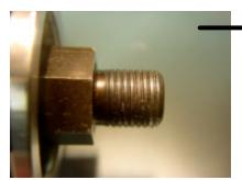
Undersize spindle threads will have a 'flattened' thread appearance
