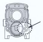
IMPORTANT! A Rotary Hammer with a cast surface crankcase at clutch screw boss REQUIRES the 45-76-0490 Clutch Tube in place. If the 45-76-0490 Clutch Tube is omitted from a cast crankcase the clutch may not slip.
