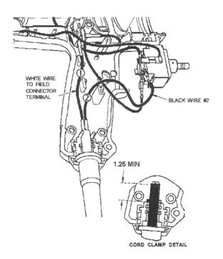
Wiring specification has been modified increasing the length of cord inserted through the strain relief, cord clamp and into the handle from .25" pass top of cord clamp to 1.25" [see illustration].
