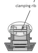
As an aid in determining the cord clamp in a tool, the 31-17-0270 Cord Clamp has the numbers '0270' molded into the clamping rib. The 31-17-0265 Cord Clamp has no markings on the rib.
